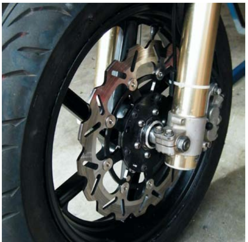
DISC ADAPTER & SUZUKI GSXR750 OR GSXR600 310MM FULL FLOATING FRONT DISC
