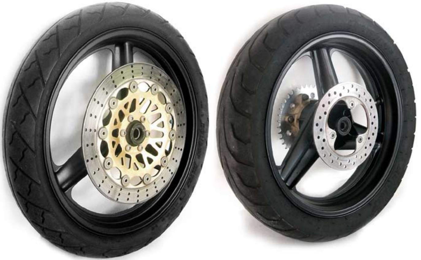
TYPICAL THREE-SPOKED SETUP, CBR250R WHEELS FRONT & REAR
